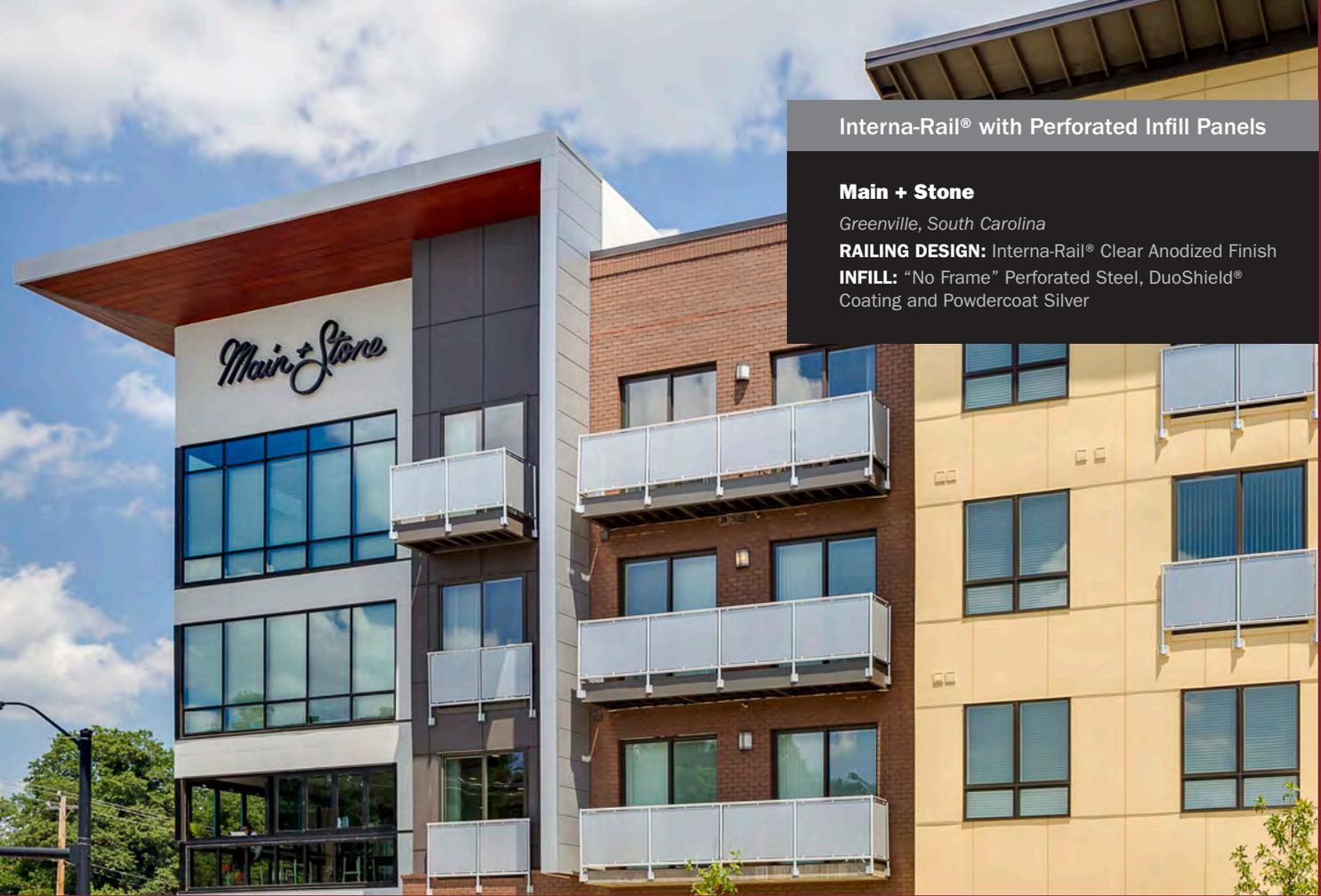
**Interna-Rail® with Perforated Infill Panels**
