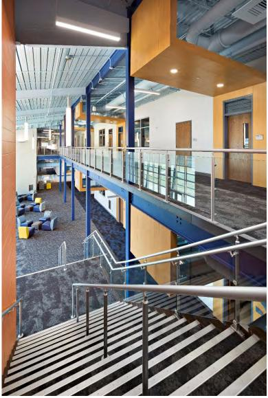
Stainless Steel VUE™ Railing System with Glass Infill
