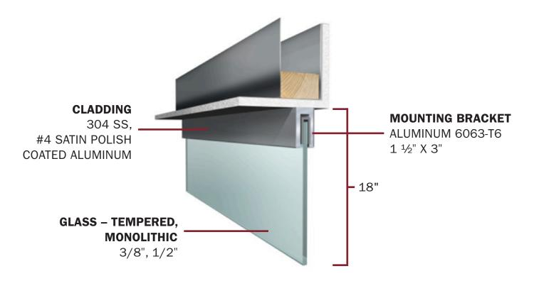
Smoke Baffles are required in some buildings to limit the spread of smoke and provide adequate egress during evacuations.
